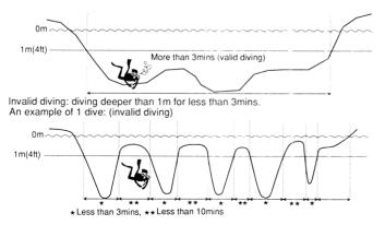
One dive: In this watch, one dive starts from the time you dive deeper than 1m (4ft) to the time you return shallower than 1m (4ft) depth. However when diving deeper than 1m (4ft) after being shallower than 1m (4ft) for less than 10 mins, the watch will record it as one continuous dive.
